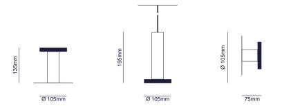
Solid alabaster disk Ø105mm and 15mm thick, attached to an oak wood cylinder Ø50mm and variable length.
